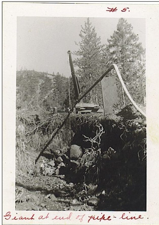
Fig. 3. Rainwater Feed Water Giant (Reproduced from F.E. Cooke, private collection, photo #5, circa 1934).
